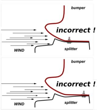
Wind could cause the splitter's damage if the bolt is not installed correctly.
