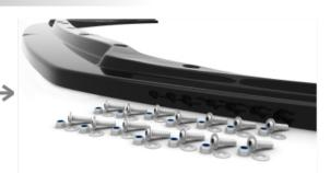
Always match the splitter to the bumper to make sure it fits before the installation.
